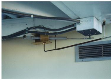
Figure 1.11: *This is the LVDT (Linear Voltage Displacement Transducer) which measures the position of the dome relative to the antenna. This is the way we know where the dome is. This transducer is located under the sidecab, and can be seen easily from the first floor. If you ever have to move the antenna off of a dome-telescope limit switch, using the hand paddle, then you'll want to place this transducer in the center of its travel.*
