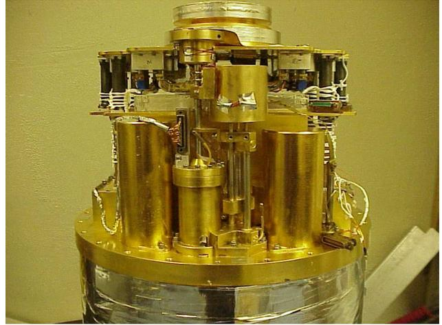
Figure 2.1: The diagram on the left is a simple schematic of the three-stage sorption refrigerator used in Bolocam. Figure taken from Bhatia et al [13]. The image on the right is a picture of the refrigerator installed in the Bolocam dewar.
