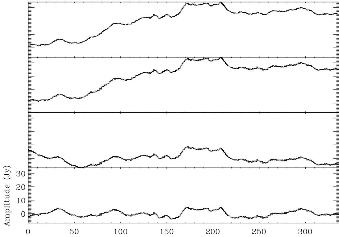
Fig. 6a.— Removal of the  $e$  and  $p$  models. From top to bottom: 1. Raw time series 2. After removal of residual 60Hz signal 3. Exponential decay function at scan turnarounds subtracted 4. A polynomial (with astrophysical source rejection) is fit to remove large-scale variations across the scan.
