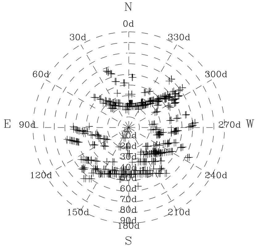
Fig. 3.— The distribution of the pointing calibration sources across the local sky in Hawaii during July 2007 (Epoch V) when the master pointing model was constructed. Note that the entire local sky is sampled, and the residual pointing RMS is valid for any point on the sky.
