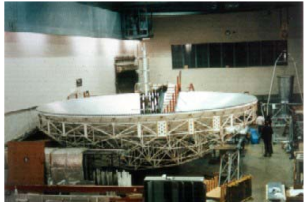
Figure 1. The submillimeter dish on an air-bearing, and under the parabolic cutter-track, in the large, thermally stable building originally constructed for work on the Palomar 200” telescope.
