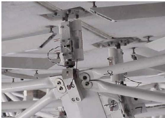
Figure 5. A view of one of the Peltier units which control the lengths of the stand-off pins. There are 88 such units on the telescope.
