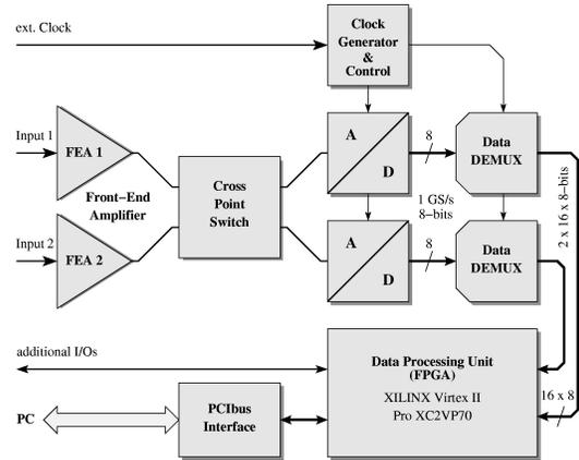
Fig. 2: Block diagram of Acqiris' AC240 digitizer/ analyzer board, the main hardware of the FFT spectrometer. By applying interleaved techniques, the two 1 GS/s 8-bits ADCs can be combined to one 2 GS/s converter. To feed the high data rate output of the ADCs (2 GBytes/s) to the FPGA, de-multiplexers (DEMUX) are used which split the two 8-bits data streams at 1 GHz to 2x16 streams at 62.5 MHz, suitable for the FPGA.
