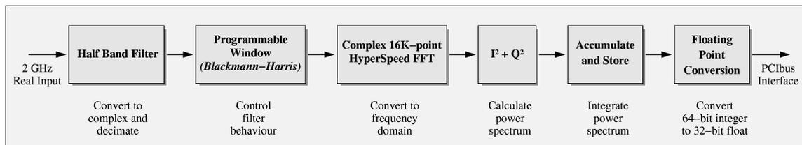
Fig. 6: Real-time FFT processing pipeline
