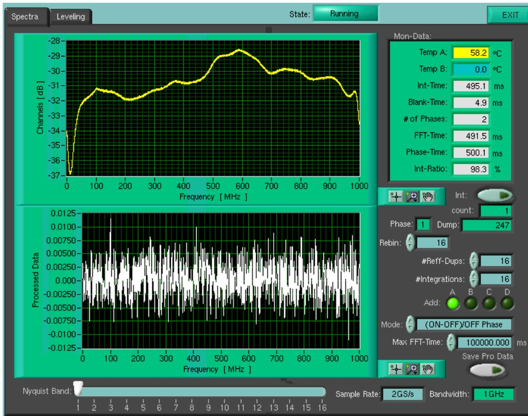
*Fig.9: Display of the LabView-GUI. In the upper panel the bandpass of the FFTS spectrum is shown, in the lower panel difference of two sequencing dumps is plotted. On the right side the operational parameters and settings are listed.*
