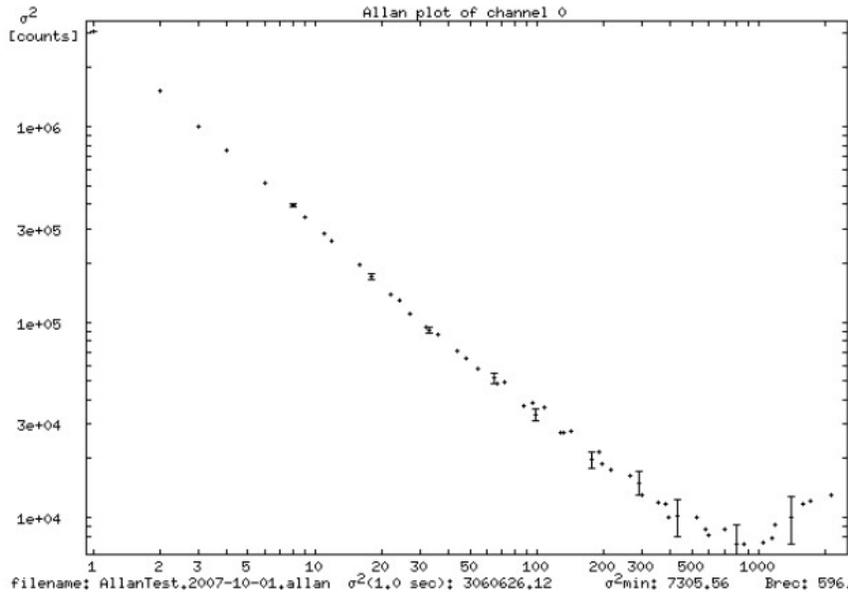
Fig.8: Spectroscopic Allan stability of the CSO-FFTS connected with the CSO-IF processor. Similar to fig.7, the variance is calculated for two 1 MHz broad channels which are separated by 600 MHz within the 1 GHz band.
