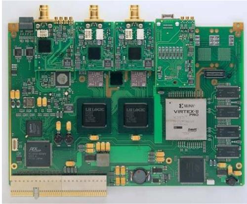
Fig. 1: Photo of the AC240 digitizer board. The AC240 is a dual-channel 6U compact PCI/XI digitizer with an onboard real time processing unit. The picture shows on the top the two analog inputs for the signal at intermediate frequency (DC-1 GHz), an input for trigger and/or clock, and the system control interface. The FPGA processing unit is visible on the right side, and the PCI bus for data output is shown at the bottom left ([www.acqiris.com](http://www.acqiris.com)).
