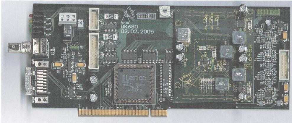
*Fig 3: Photo of the IRIG-B board, as developed in the DigitalLabor of the MPIfR*
