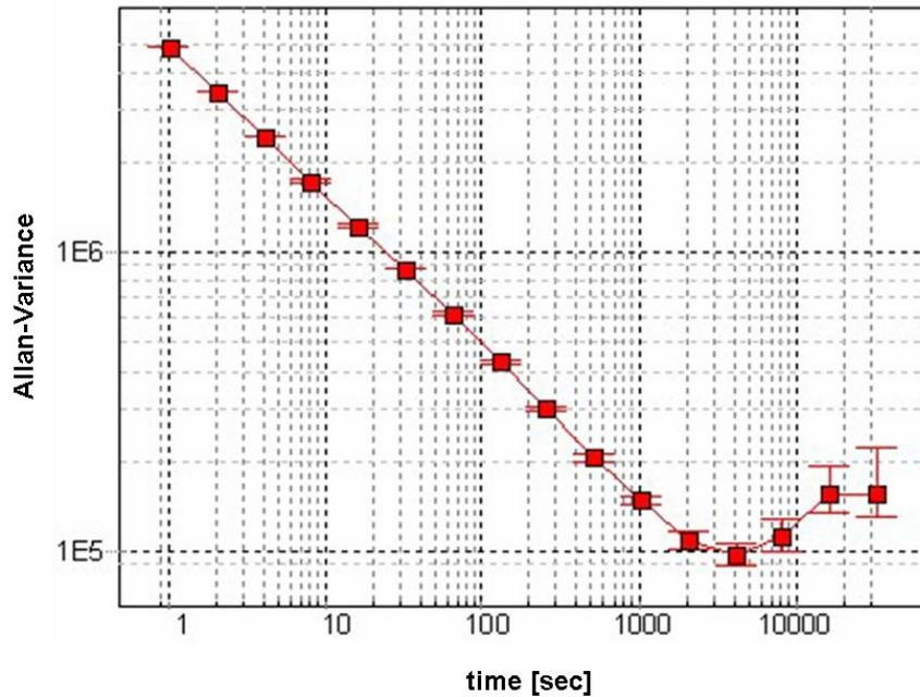
Fig.7: The excellent stability of the FFTS is illustrated in this Allan-Variance-Plot. The signal of a noise source (0–1 GHz) was integrated and processed in the FFTS. The spectroscopic variance between two 1 MHz broad channels, separated by 600 MHz within the band, was determined to be stable on a timescale of ~4000 s.
