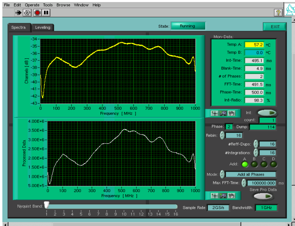
Fig.1: Display of LabViewMon: In the upper panel the bandpass of the FFTS is shown in a logarithmic level y-scale and a linear frequency (x-)scale (DC to 1 GHz). In the lower panel, the bandpass is plotted on a linear scale for both axis. In the right column the operational parameters (blank/sync time, FPGA temperatures, etc.) and the settings for the FFTS are listed. Note: The CSO-FFTS version provides only one bandpass (1 x 1 GHz), therefore only one FPGA temperature is displayed!
