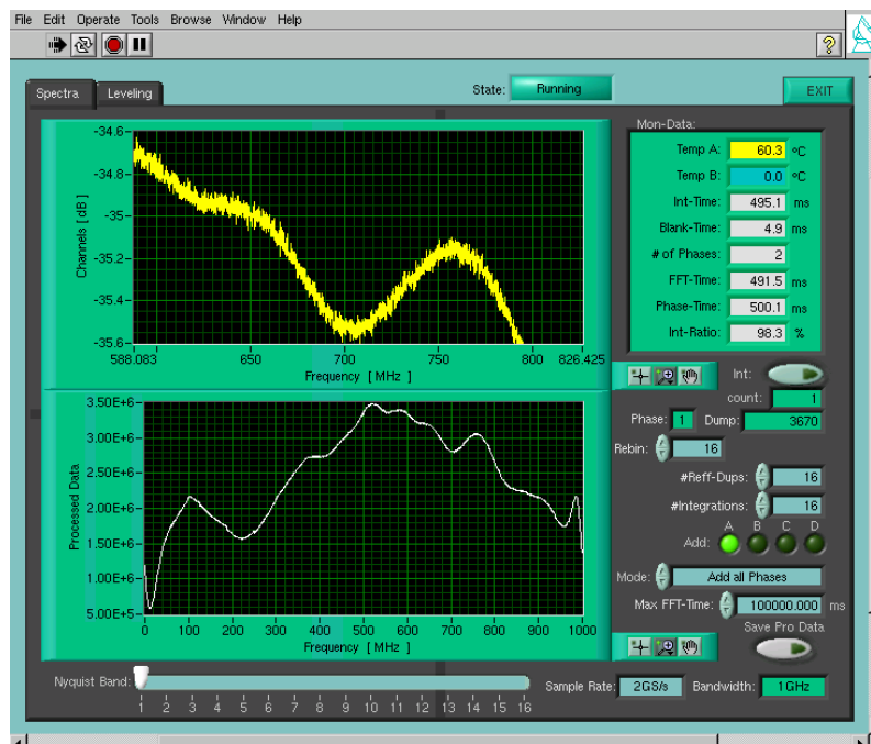
Fig 6: The upper panel shows a subsection of the bandpass after zooming-in on the y-scale. With this smaller span a more detail view of the bandpass structure is possible.
