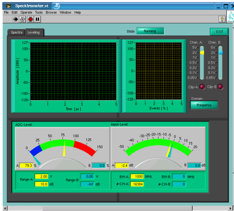
Fig 7: The Level-Display: The upper panels are only used for sophisticated debugging purposes. Therefore they are not described in this manual. The lower panel shows the leveling for the FFTS (yellow). The chart in the left corner at the bottom line shows that the FFTS level is around 75% ADC full-scale, which corresponds to an input level of \sim -3 dB.
