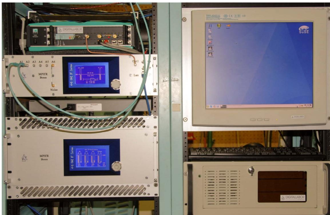
Fig.A1. The CSO-FFT/IF spectrometer as installed in the backend room at the CSO. The left panel shows the (from top), the Acqiris FFT board, the IF processor and the IF power supply. To the right: the FFT control computer with its flat screen.
