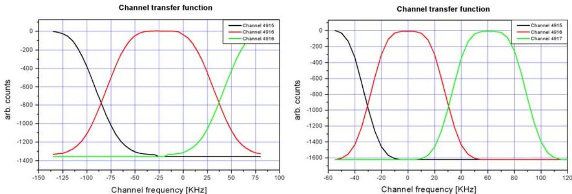
Fig.7. The spectral response of the CSO-FFT/IF as measured for both the 1000 and the 500 MHz core. The response functions are identical.
