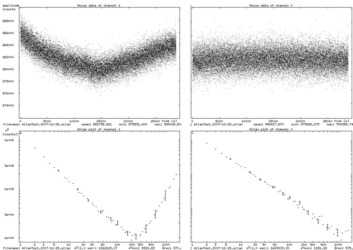
Fig.1. Measurement of the continuum (channel # 200) and spectroscopic (# 800 vs. 200) Allan variance of the FFT/IF spectrometer as installed at the CSO. Data were taken on the integrated 4-8 GHz noise source. The variance is calculated for two 1 MHz broad channels, separated by 600 MHz within the 1 GHz video band. Total power (continuum) AV times are  $\sim 250$  sec, the spectroscopic AV time is  $\geq 1000$  sec.
