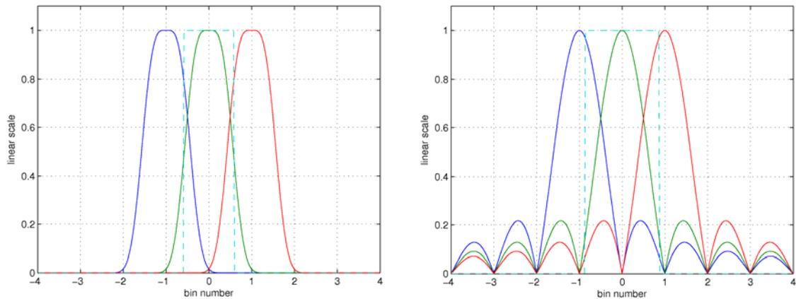
Fig.6. Simulation of the superior spectral response function of the FFT WOLA core, compared to an autocorrelator, which equivalent noise bandwidth is 1.7 times the channel spacing.
