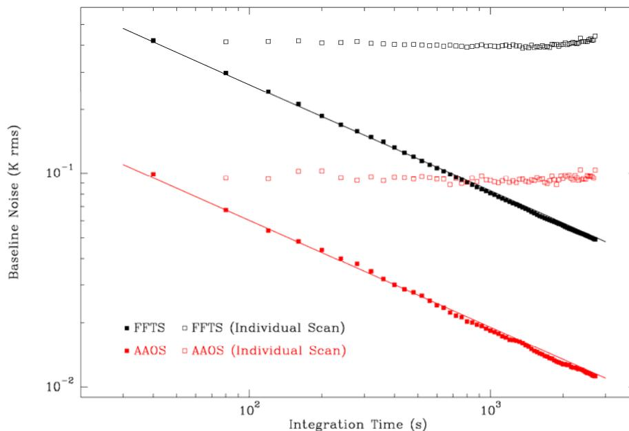
Fig.9. Noise of the cumulated spectra of a 46 min (on-source) long CO(2-1) integration towards o-Ceti, using the side cab 230 GHz receiver (FFTS: black dots, AOS: red dots). Open dots display the noise of the individual scans, reflecting unstable sky conditions.
