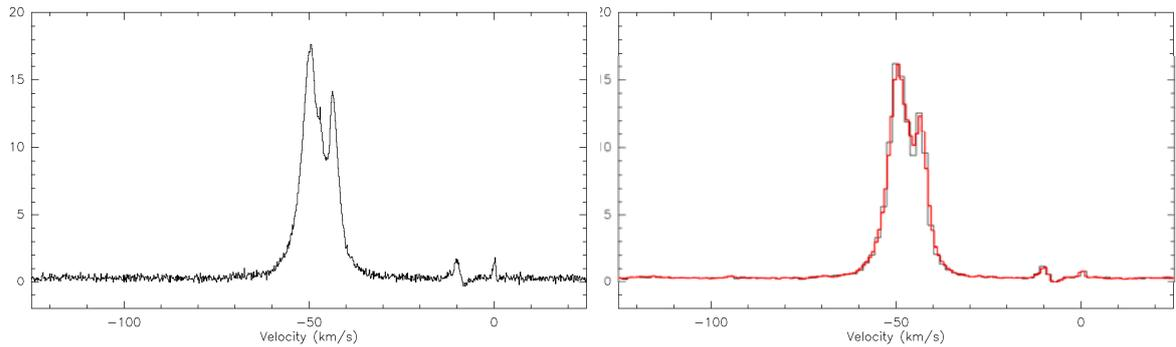
Fig.4. First FFTS spectrum observed in wobbler mode (300" throw, 0.5 Hz), during rather limiting atmospheric conditions (8 mm H<sub>2</sub>O). The spectrum to the left displays the FFTS data in nominal resolution (120 kHz). In the right panel, this spectrum has been box-smoothed to the nominal resolution of the AOS (1.2 MHz), superimposed in red. The data agree pretty nicely, differences are likely due to the different effective resolutions/spectral responses of the two backends.
