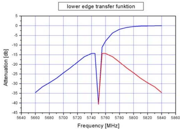
Fig.10. Transfer function of the spectrometer in the 500 MHz mode: suppression is good, the lower half of the IF band can be used up to -230 MHz or more, unless very high rejection is required (220 MHz for 20 dB). The performance of the filter at the upper band edge has not changed (Fig. 8).
