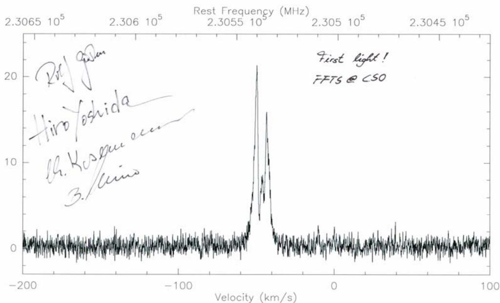
Fig.2. **First-light spectrum** with the CSO-FFTS & IF processor, recording a 1 GHz wide spectrum towards W3(OH). Frontend: side cab 230 GHz Rx, with the CSO up-converter. The integration time of this total power observation was 0 sec, the reference position was at 600" AZ (afterwards, a pointing offset of ca. 10" was determined).
