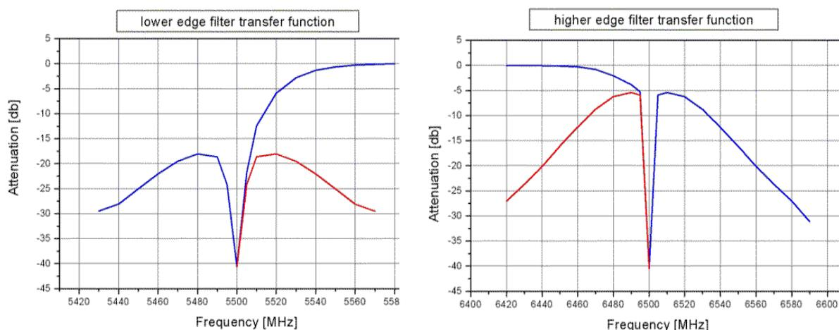
Fig.8. Transfer function of the FFTS/IF-processor. The lower half of the 1 GHz IF band is limited to -480 MHz, the upper half to +440 to 470 MHz for 20 (10) dB suppression, respectively.
