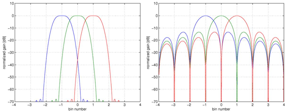
Fig.5. Frequency response of the FFT channels for the WOLA core (left panel). The response was confirmed with a narrow (few kHz) line that was injected via a power splitter (combining the
