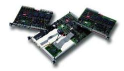
VME and VXI cards all use common design. The main difference is that the VXI modules do not include the P2 bus connector. The VXI-C module is functionally identical to the VXI-B module, the only difference being the length of the module.
