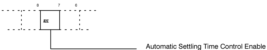
Figure 8: CONTREG Automatic Settling Time Control
