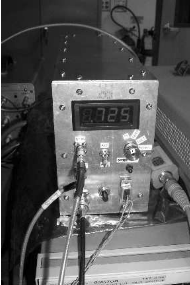
Figure 4: Photograph of assembled IF amplifier module including active temperature controller electronics.
