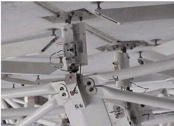
Figure 2a. TEC Assembly Installed on Primary Standoff
