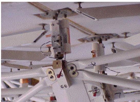
Fig. 2a. TEC Assembly Installed on Primary Standoff
