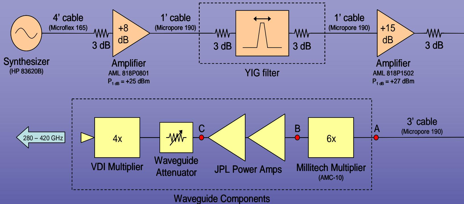
Prototype synthesized LO system tested on telescope
